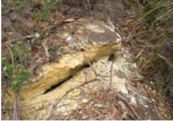
Alleged minor [upsidence] cracking claimed to have no effect on East Wolgan Swamp (Photos: C. Jonkers, 2008)
