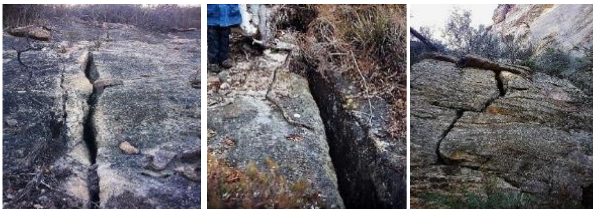
Photos: State Mine – cliff falls and surface fractures in the State Mine Airshaft No. 3/Lost City area – 17 July 2019
