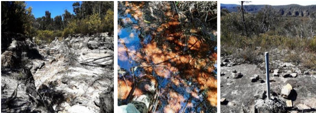
Photo 80-82: Panel 314 – Severe channelisation, erosion, rusty-red discoloured water, old mine subsidence peg
